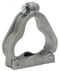
Aluminium single two bolt trefoil cleats are suitable for cables in trefoil groups from cable diameters 24mm to 76mm. They can be used with all types of cable routes, and are suitable for use at a maximum fault level of 30kA rms. Single fixing, with a plain finish which is suitable for indoor dry, industrial use, or in outdoor unpolluted areas.
